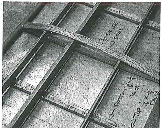
Complete airfoil by placing \frac{1}{8} -inch-thick balsa strips on top of spars. Soak strips in water so they will bend easier.
