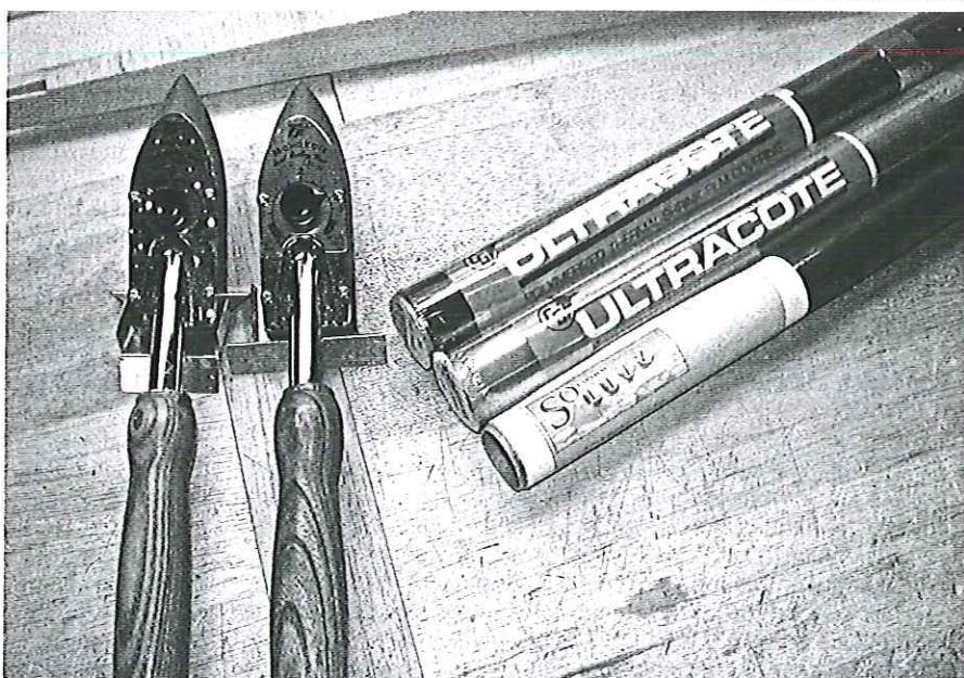
As text explains, Bob uses two identical heating irons to apply covering.
